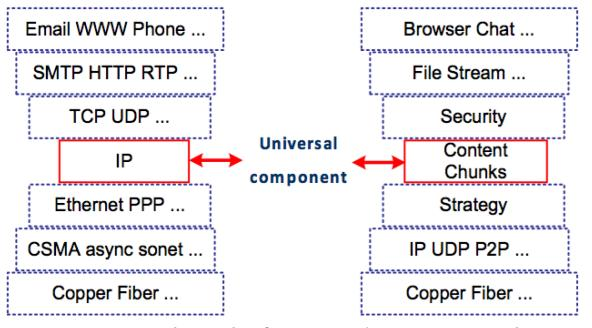
CCN[1] allows users to focus on the data's names rather than the location where that data is to be retrieved. This is realized through replacing current forwarding mechanism of IP addresses with a mechanism based on named contents
