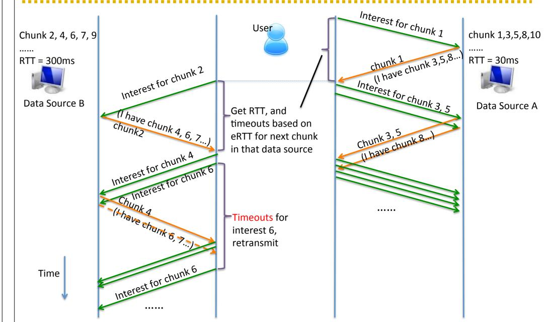
User wants to retrieve a content segmented in 10 chunks which stored in two separate Date Sources In this topology:
